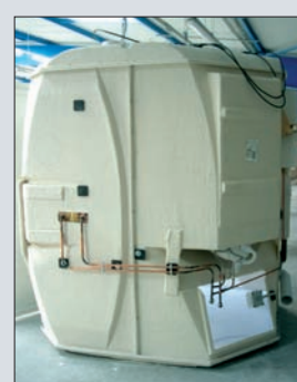
Rear view of the Altor pod. Plumbing connexions right next to the removable panel.
