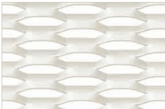
Maglia/Mesh: FILS 21 45 x 15 (13,4) - 5 x 1,5 mm Acciaio al carbonio Sendzimir verniciato/Powder coated pre-galvanized steel
